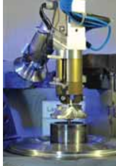
Forged-milled compressor wheel production
