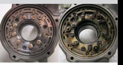
Original Garrett® VNT™ turbosnozzle assembly made from top quality materials. Remanufactured VNT™ turbos-nozzle assembly made from reused components.
