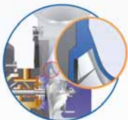
Compressor wheel with extended tip technology
